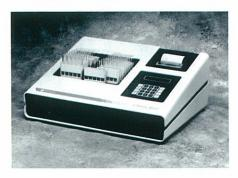
ests for Glucose/Fructose, Acetic Acid, Malic Acid, Volatile Acid, Alcohol and other tests from 340 to 650 nm.
