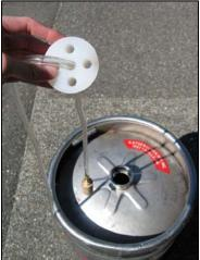
3) With the regulator pressure set to 10 psi, and the **AIR flowmeter** reading 20 liters/minute (which corresponds to 15 L/min of argon), it took 5 minutes for the % oxygen at the top of the keg headspace to fall below 0.5% O<sub>2</sub>.
